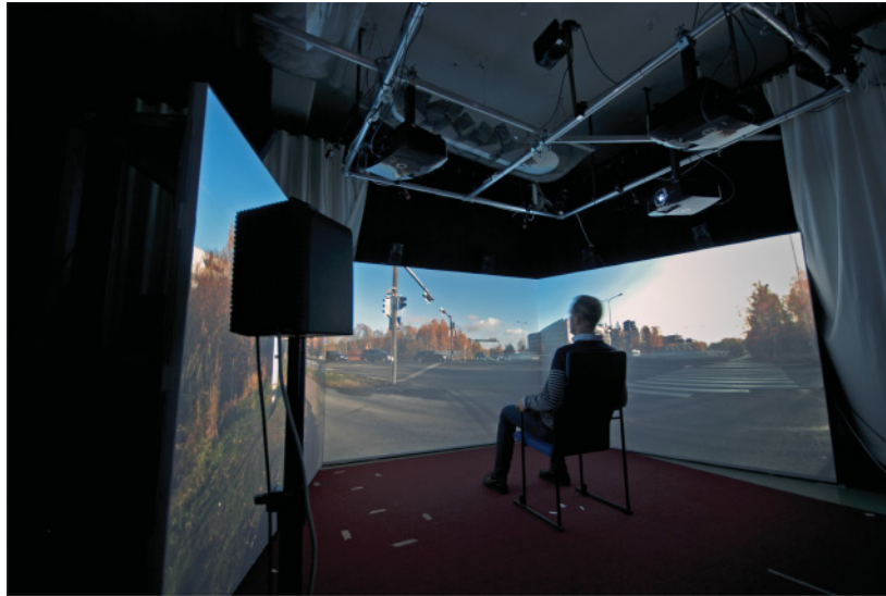
Fig. 2. View of the audiovisual environment with a participant seated in the observation position. The projectors can be seen overhead of the participant. The projection screens cover the frontal loudspeakers.
